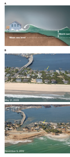
FIGURE 9.17 Storm surge (A) not only inundates areas normally above high tide, but also brings breaking waves that demolish structures. Photo (B) of Mantoloking, New Jersey, showing the effects of storm surge and waves associated with Hurricane Sandy in 2012. Arrows mark the same house that appears in both images. Notice the destroyed houses and roads and extensive beach erosion. Also note the large volume of sand that was deposited on the back side of the island. (a) (both) USGS
